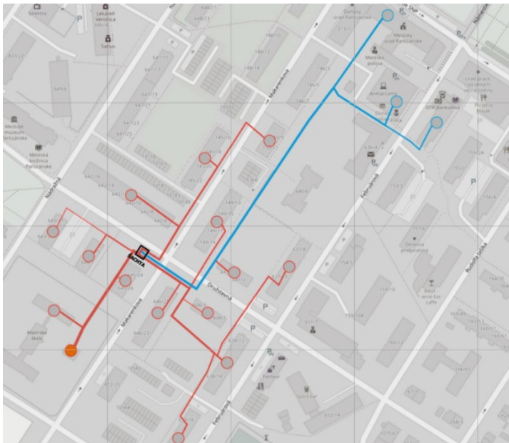
Fig. 29: New distribution branch from the shaft at building 645 (blue - connected section and connected objects PK 18, PK Alfa and PK 13) 50
